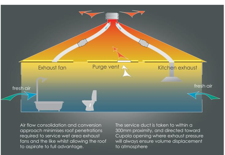
This facility provides the option in non dedicated venting of individual rooms, with the use of purge vents that can be opened and closed from trickle to full flow displacement. See Purge or Displacement venting.
