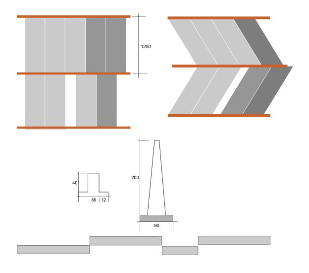
Insert panels can be either proprietary items or panels designed to specific performance values as required. Layout can be wall to wall, island, fragmented or peripheral with grid patterns being within the 1200 x 1200 in increments of 300, 400, or 600mm Three dimensional disposition is also available with the use of recessed cradles to a height of 100mm
